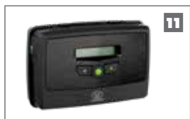
G-ULTRA The ultimate GSM solution for monitoring and activating the operator via your mobile phone
